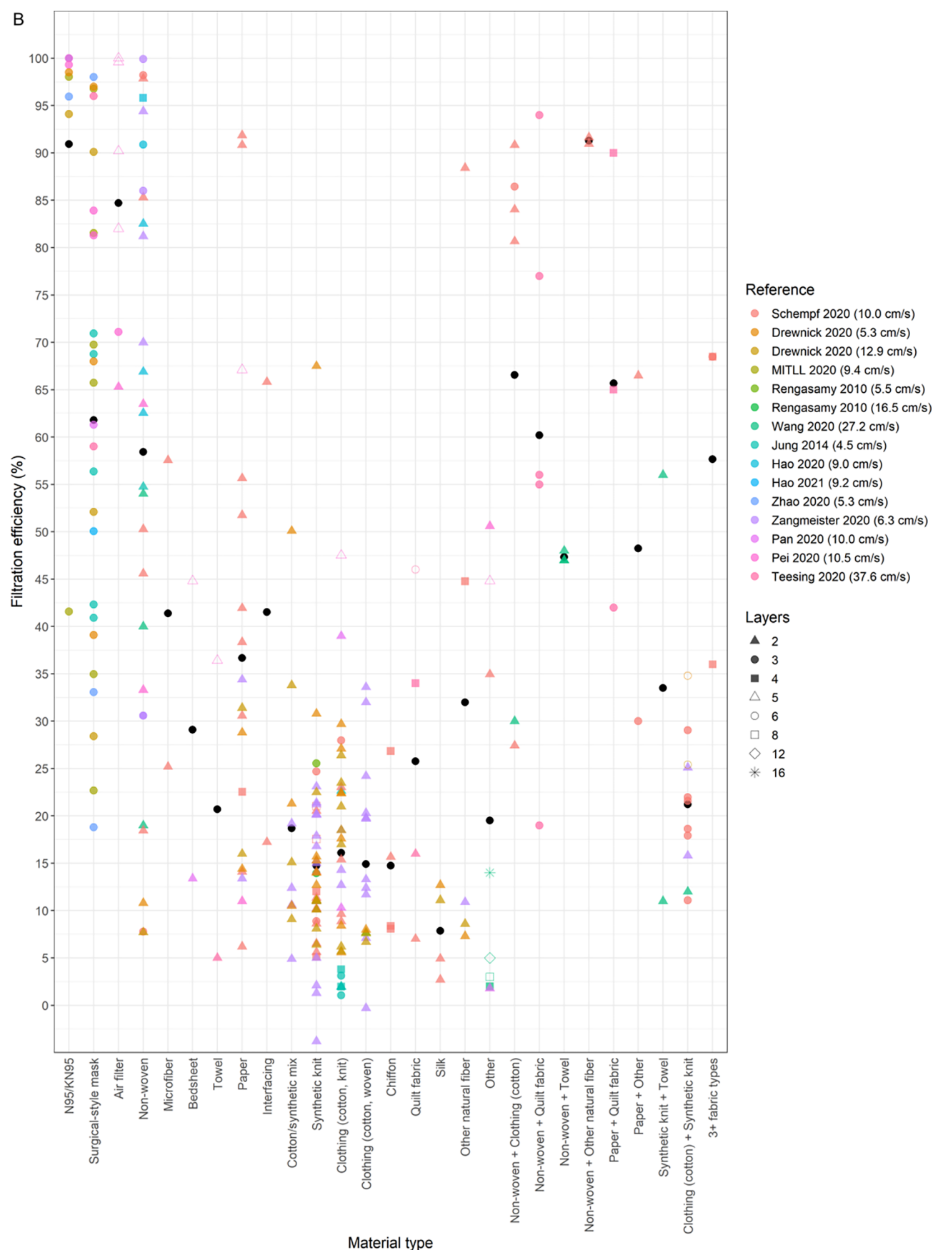
Figure 5. Filtration efficiency for (A) single and (B) multiple layers of various materials. Combinations of fabric with only one data point were omitted for clarity. The black dot indicates the mean filtration efficiency for each material type.
