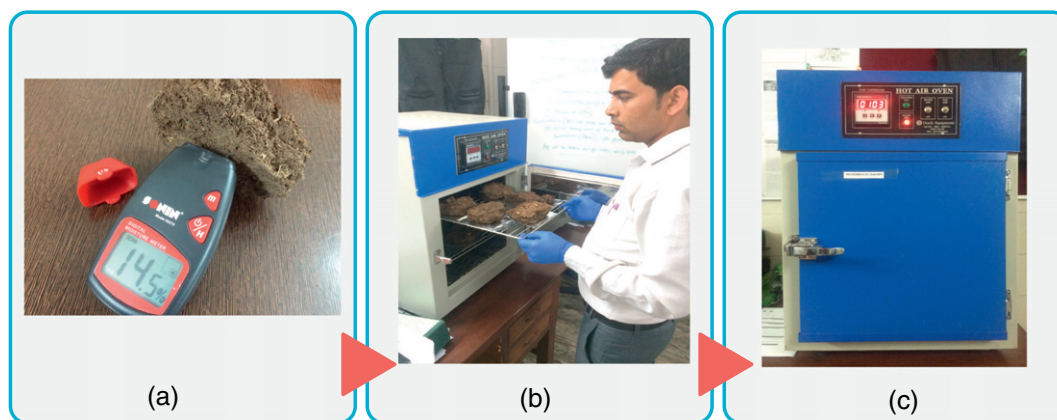
Fig. 3. Moisture measurements: (a) moisture meter with sample, (b) sample arrangement in convection oven and (c) convection oven.
