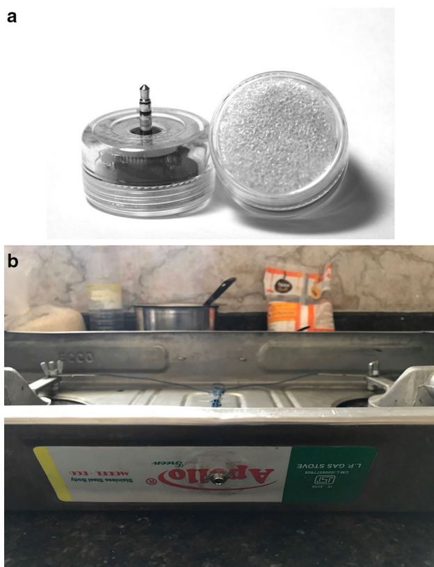
Figure 2. a-b The Pink Key Sensing System. a The Pink Key meal-counting datalogger. Approximately 1.5" diameter and 0.75" tall with a 0.5" 3.5-mm headphone jack for mounting on the stove. b The mounting location for the PK on the front of a two-burner LPG stove (shown flipped over, resting on its burners). Also visible is the location of the two diodes connected to the bolts near the burners for measuring temperature changes on the stove.
