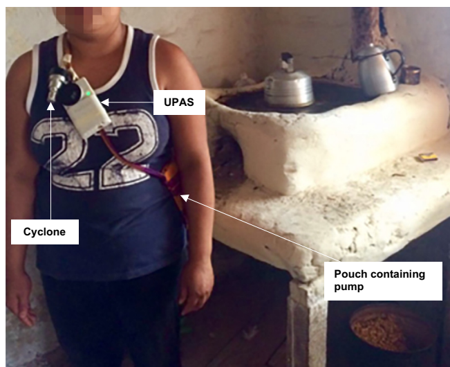
Fig. 1. A participant wearing both the UPAS and the typical pump and filter gravimetric samplers. Note that both the cyclone from the pump and filter setup and the UPAS are approximately located near the participant's breathing zone.
